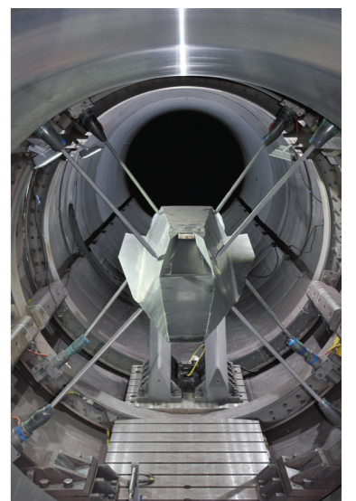
JF12试验模型-吸气式高超声速飞行器内外流一体化性能试验 A test model of JF12 - A hypersonic air-breathing vehicle for the integration performance study on inner/outer flow interaction
